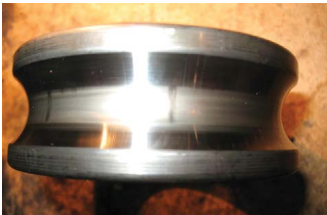
Figure 2. Bearing race exhibiting a "frosted" appearance.
