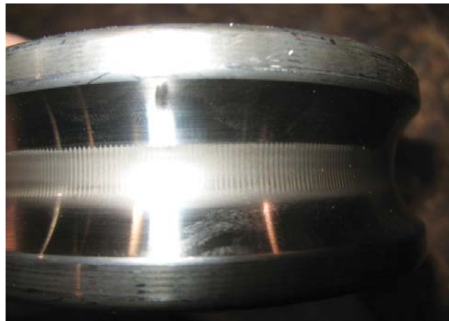
Figure 3. Bearing race exhibiting "fluting".
