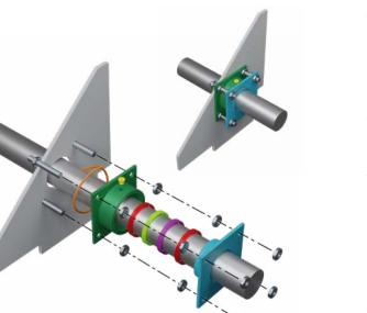
**Theory of Operation** — The stuffing box is sealed to the fan housing with PTFE joint sealant for a gasketing material. The packing materials are a flexible graphite split ring and a lantern ring sandwiched between two carbon yarn anti-extrusion rings. The outside hex nuts force the outside packing plate into the stuffing box, expanding the graphite rings to provide a leak tight seal. A pressure purge tap is provided to insure that all leakage will be the purge gas.
