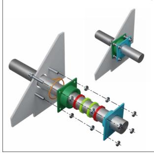
**Theory of Operation** — The stuffing box is sealed to the fan housing with PTFE joint sealant for a gasketing material. The packing materials are two flexible graphite split rings sandwiched between two carbon yarn anti-extrusion rings. The outside hex nuts force the outside packing plate into the stuffing box, expanding the graphite rings to provide a leak tight seal.
