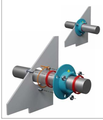
Theory of Operation — The sealing action is provided by two lip type seals placed back to front within a seal housing with a layer of grease between them. The grease reservoir may be maintained using the grease fitting in the seal housing. The contact is between the seal inner lip and the circumference of the fan shaft.
