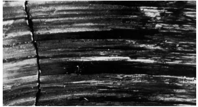
Figure 23. Fretting Corrosion on Bearing Bore
