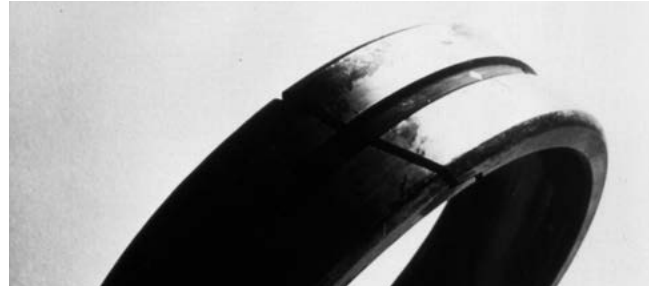
Figure 26. Pits Caused By Electrical Current
