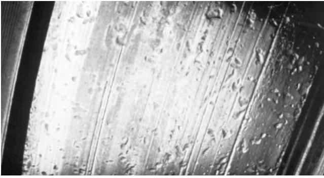
Figure 13. Severe Particle Denting
