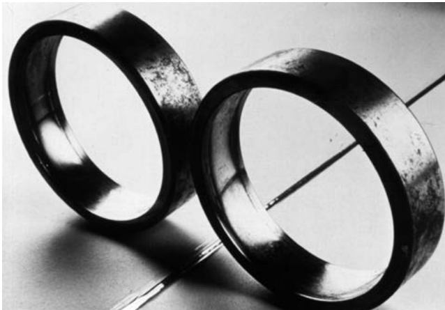
Figure 21. Two Load Zones on the Outer Race
