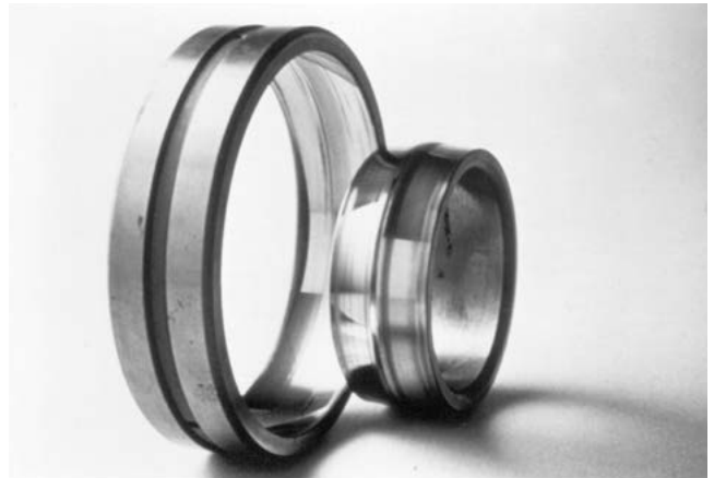
Figure 12. Highly Polished Surfaces Due to Inadequate Lubrication
