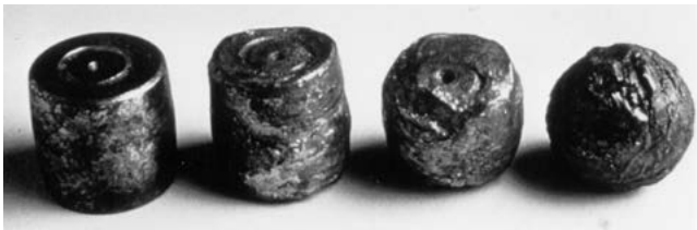
Figure 9. Damaged Spherical Bearing Rollers
