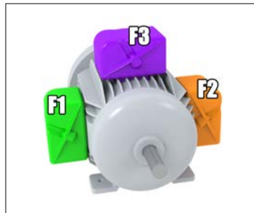
Conduit Boxes (viewed from drive side of motor, looking at motor shaft)
