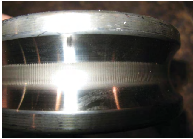
Figure 3. Bearing race exhibiting "fluting".
