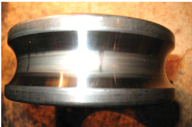
Figure 2. Bearing race exhibiting a "frosted" appearance.
