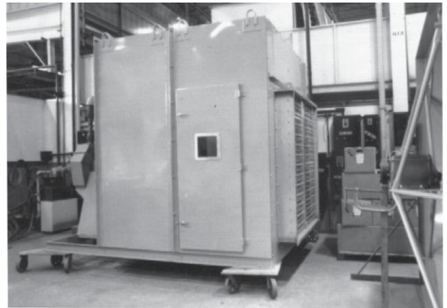
*A gas-fired air make-up unit on the test stand. All units are tested before delivery.*
