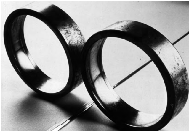
Figure 21. Two Load Zones on the Outer Race
