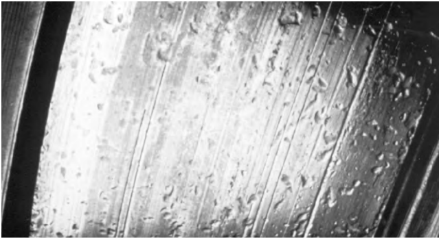
Figure 13. Severe Particle Denting
