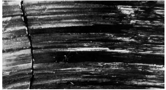
Figure 23. Fretting Corrosion on Bearing Bore
