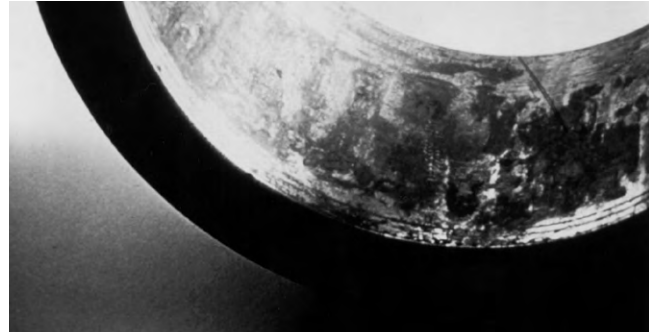
Figure 24. Cracked Inner Race
