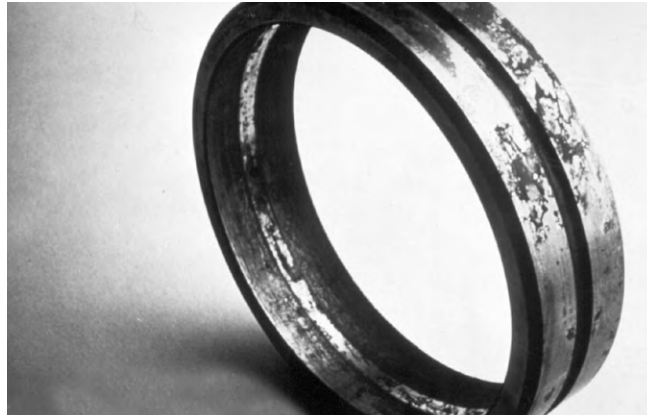
Figure 15. Bearing Roller with Rusty Ends Due to Moisture in the Lubricant
