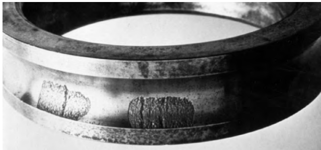
Figure 21. Two Load Zones on the Outer Race
