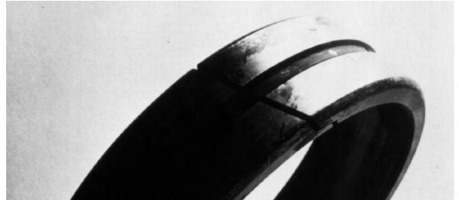
Figure 26. Pits Caused by Electrical Current
